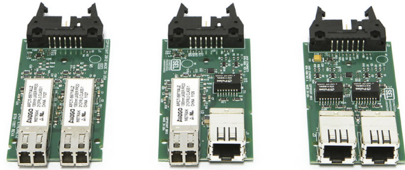
Figure 13 Ethernet Communications Cards
